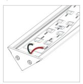
4 Install the LED strip on the fixture surface.
