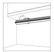
7 Connect the wires and install the fixture into the mounting brackets.
