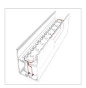
"Electrical connection must be made from both sides for fixtures longer than  $2500\mbox{mm}$
