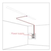
power supply and then run the wires to the location of the light fixture.
