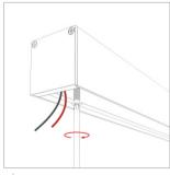
Run the wires through the hole, then secure the fixture into the surface.
