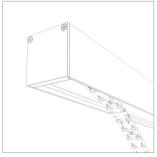
5 Install the LED strip on the fixture surface.
