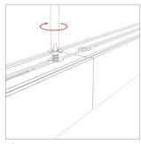
Drill in the connection piece where both fixtures connect
