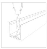
2 Drill a hole into the fixture for low voltage
