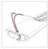
Install the LED strip on the fixture surface.
